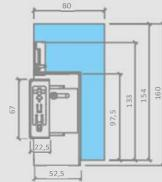
Fundo Discreto attachment element, channel length 1.100 mm
