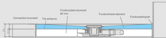
Fundo substructure set, point drain horizontal, substructure height 90 mm
