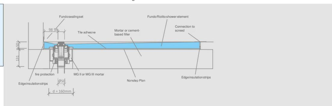
wedi Fundo® channel drain Mini Max ▪ horizontal, extra flat, DN 40
