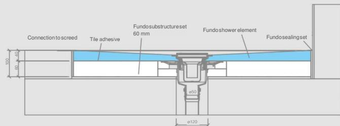
Fundo substructure set, point drain Mini Max, substructure height 60 mm
